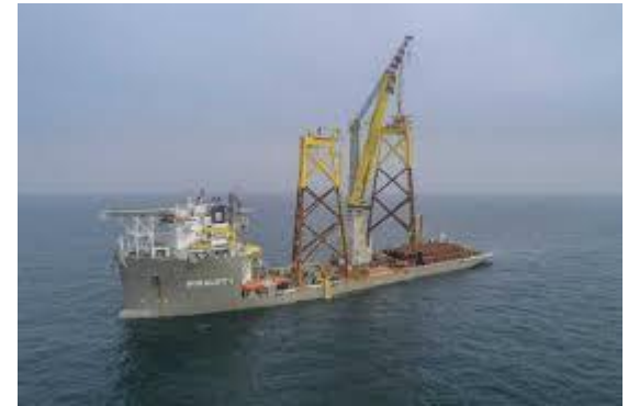
Floater "Bokalift 1" Max. 3 foundations
